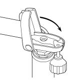
**5** Pivot the handlebar assembly upright.
